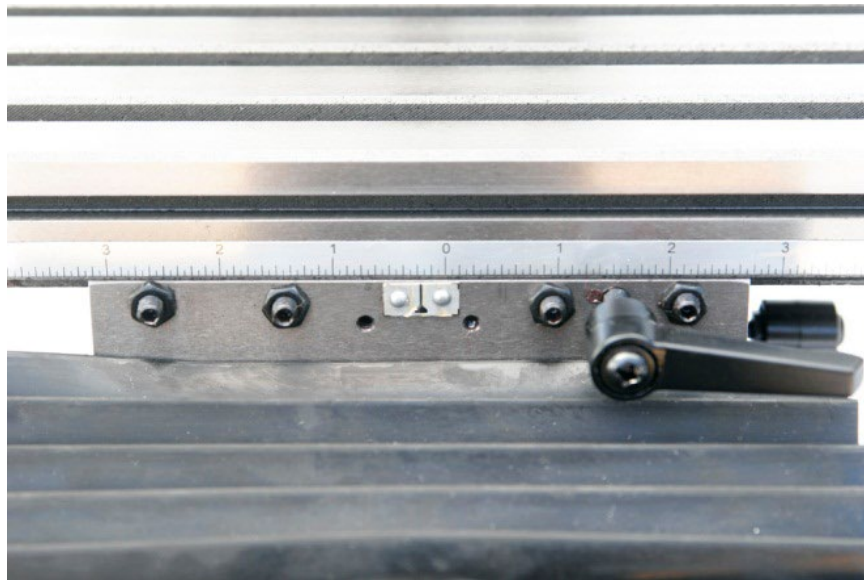
X-axis gib adjusting screws
